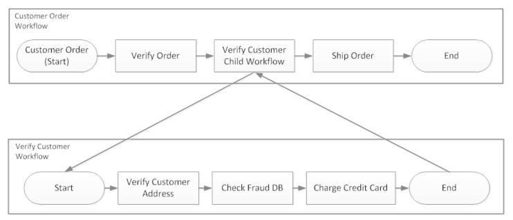
Multiple workflows could create child workflow executions using the same workflow type. For example, the Verify Customer child workflow could also be used in other parts of an organization. The events for a child workflow are contained in its own workflow history and are not included in the parent's workflow history.
