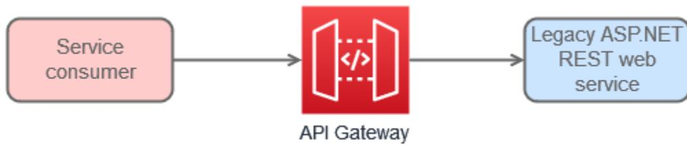
When the API Gateway proxy is in place, you can create and deploy the modernized service on AWS by using Amazon ECS, for example, to achieve a highly scalable and available service. When the proxy and newly modernized service have been created and tested, you can reconfigure the API Gateway endpoint to point to the modernized REST API for its implementation.
