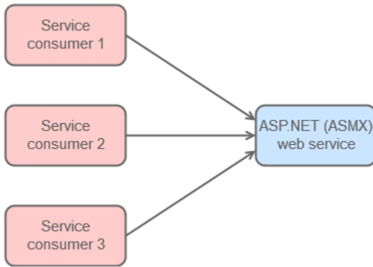
Because these consumers call the ASMX service by using the SOAP protocol, replacing the ASMX service with a REST API would cause these consumers to break. Furthermore, refactoring the ASMX service to a REST API while you convert the system from a monolithic architecture to microservices will most likely involve remodeling the system behavior and domain model. This is likely to create additional breaking changes for consumers.
