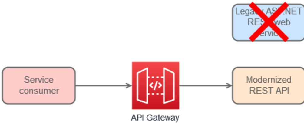
If the newly modernized service has an API contract that is different from the legacy proxy contract the consuming systems depend on, you can use API Gateway's data transformation feature. Incoming API requests that are structured using the legacy system's schema can be mapped and transformed to the new service's contract.
