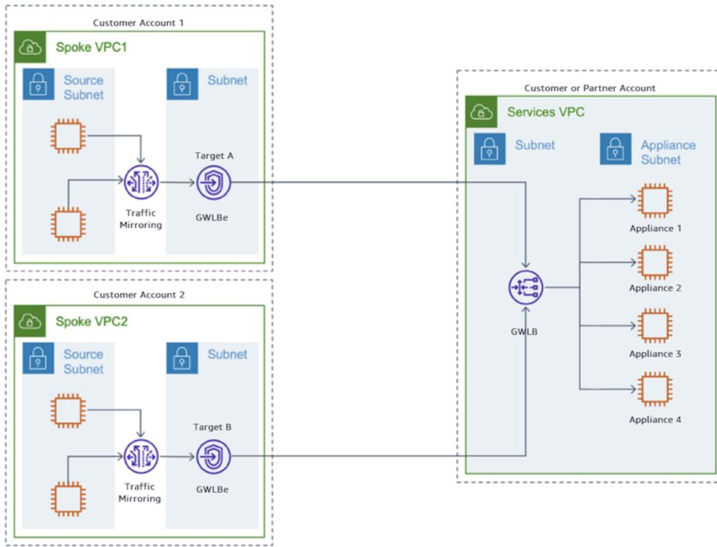
Consider the scenario where you want to mirror inbound TCP traffic on an instance and then send it to a Gateway Load Balancer using a Gateway Load Balancer endpoint. You need the following Traffic Mirroring entities for this example:
