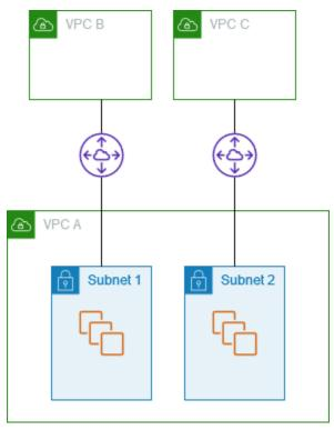
The route table for subnet 1 uses VPC peering connection pcx-aaaabbbb to access the entire CIDR block of VPC B. The route table for VPC B uses pcx-aaaabbbb to access the CIDR block of subnet 1 in VPC A. The route table for subnet 2 uses VPC peering connection pcx-aaaacccc to access the entire CIDR block of VPC C. The route table for VPC C table uses pcx-aaaacccc to access the CIDR block of subnet 2 in VPC A.
