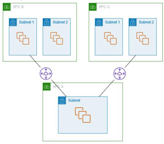
Use this configuration when you have a central VPC that has a single set of resources, such as Active Directory services, that other VPCs need to access. The central VPC does not require full access to the VPCs that it's peered with.
